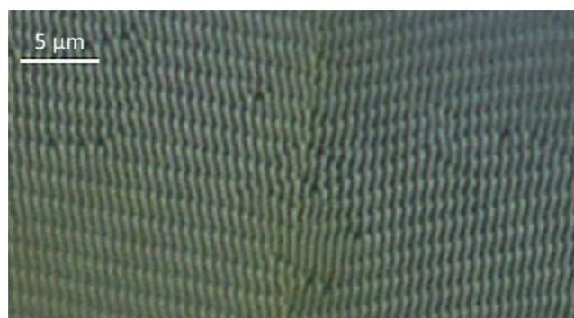
Fig. 12 Photomicrographs of undulating 9004 soapy streaks on MoS<sub>2</sub> at  $T_{AC} - T \sim 6.8^\circ\text{C}$  exhibiting two distinct chiral domains. This image has been slightly contrast enhanced to aid the reader. The  $5 \mu\text{m}$  scale bar is oriented perpendicular to the easy axis.
